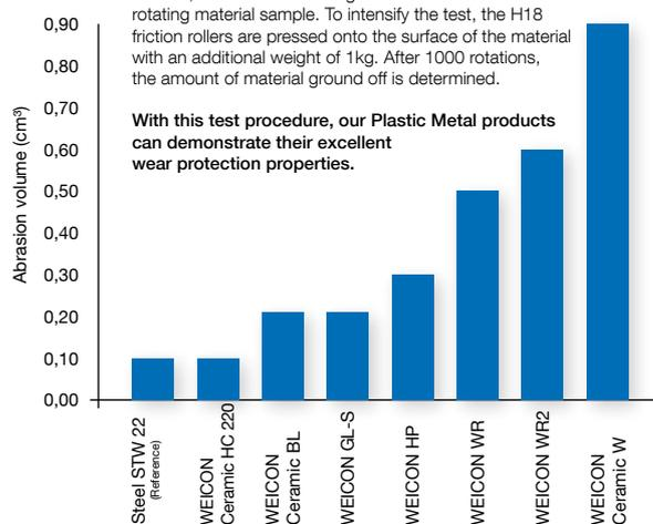
With this test procedure, our Plastic Metal products can demonstrate their excellent wear protection properties.
