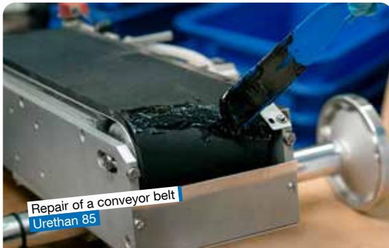
Repair of a conveyor belt
