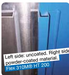
Glued and (subsequently) powdercoated plant tubs.
