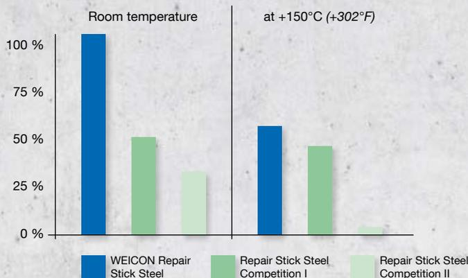
Adhesive strength of Repair Stick Steel
