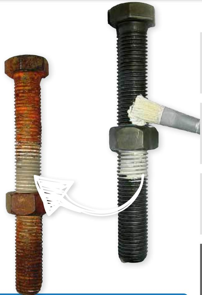
Due to the special formulation and the very fine grinding of the solids contained in WEICON Anti-Seize, irregularities in the protected surface are completely filled – even to a layer thickness of only 12 µm. Only a perfectly sealed surface guarantees a reliable protection against corrosion. An additional sealing effect thus results for special applications, such as flange connections.
