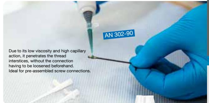
Due to its low viscosity and high capillary action, it penetrates the thread interstices, without the connection having to be loosened beforehand. Ideal for pre-assembled screw connections.
