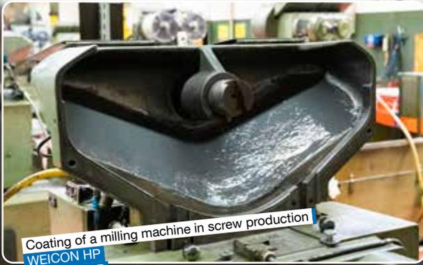
Coating of a milling machine in screw production
