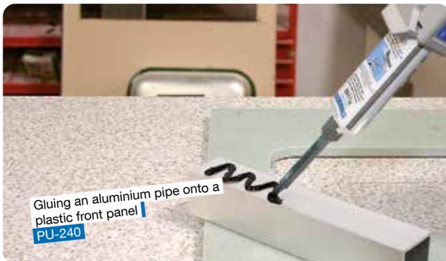
Gluing an aluminium pipe onto a plastic front panel
